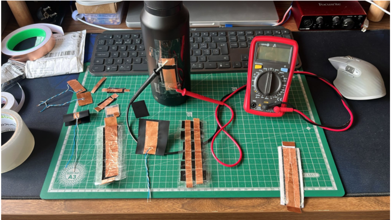
Figure 48: Velostat sensor prototypes developed during tests
